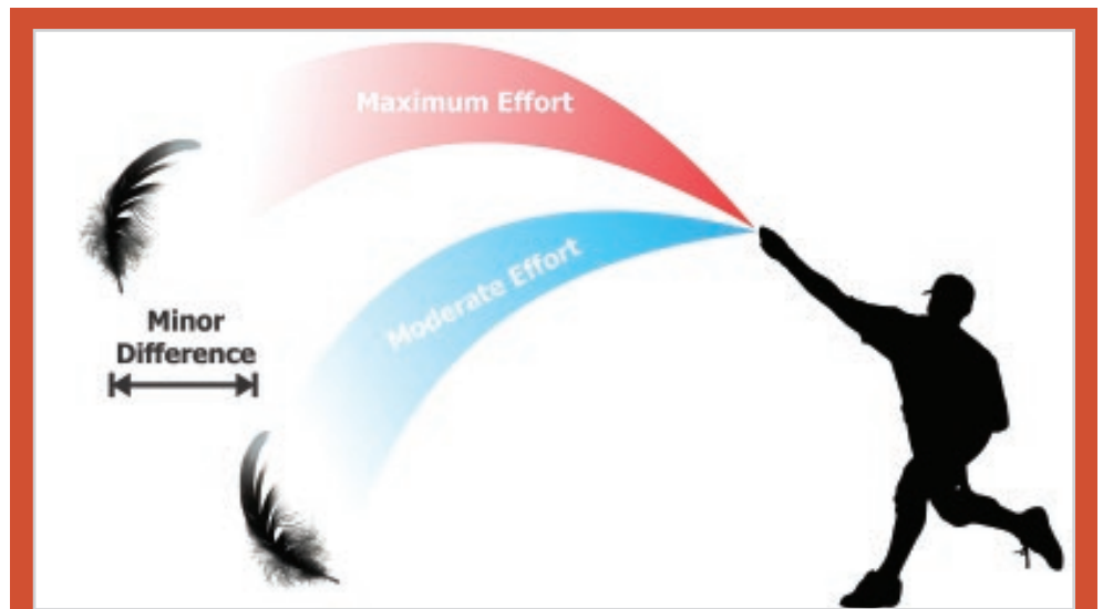
Imagine throwing a feather. Now imagine throwing it as hard as you can. It may travel a little farther, but not much relative to the extra effort. This is the primary reason for the "air" in air-assist spraying. Graphic and caption from Airblast 101.
